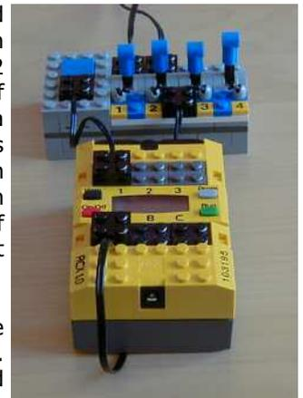
With this system up to twelve points can be run off one RCX. The duration control provided by the RCX should prevent unfortunate motor mishaps. I am thinking about modifying the program to include a reset step so that only the first button push operates the motors. Two other advantages of this design are several points can be switched at the same time and that the next point change can be set in advance.
